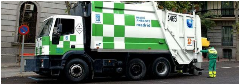
Large gas RCV
